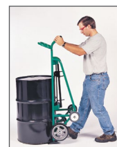
2. Tip frame against drum to engage hook.
